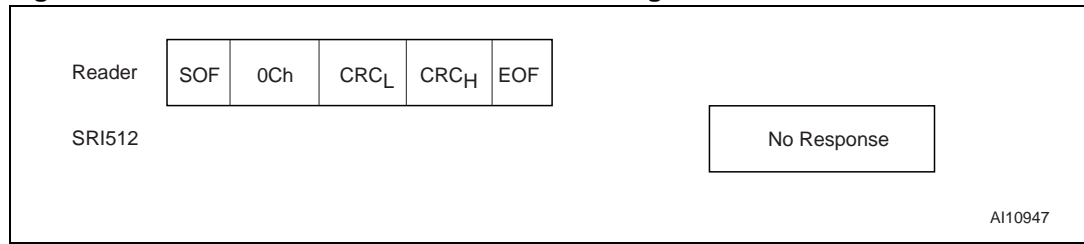
Figure 61. READ_BLOCK frame exchange between Reader and SRI512
